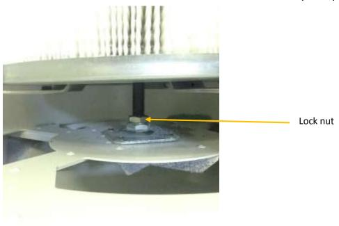
3. screw the plate of the filter clockwise completely to the bottom
